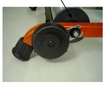
4) Adjust the gap between the magnet bar and the rear roller drums so there is a slight gap. Adjust by loosening the nuts on both axle ends and sliding each side. Sometimes a thick card can be used to help adjust the gap.
