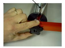
2) Install the resistance unit to the REAR roller drum so that the magnetic bar is behind the rear drum, and the black knob is behind axle on the RIGHT REAR side of the roller drum.
