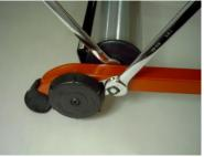
6) Make sure that you maintain a gap between the magnet bar and the rear aluminum drum after nuts are tightened.
