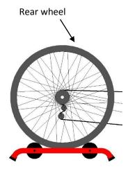
If the tire isn't well centered on the drums, adjust the alignment so that when you spin the rear tire, it stays close to the center of the drums.
